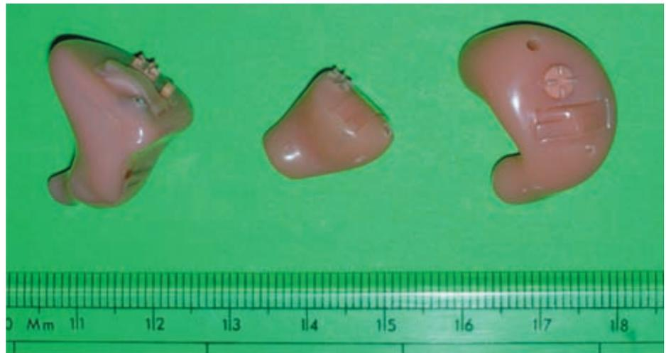
**Figure 4.1** In the ear (left and right) and in the canal (centre) hearing aids.
